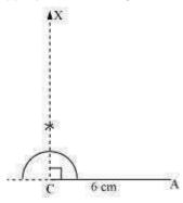
(iii) Taking point C as centre, draw an arc of 6 cm radius to intersect CX at point B.
