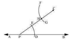
(iv)Adjust the compasses up to the length of DE. Without changing the opening of compasses and taking H as the centre, draw an arc to intersect the previously drawn arc FG at point I.
