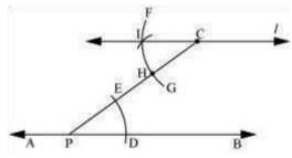
This is the required line which is parallel to line AB.
