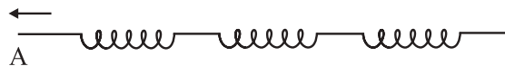
Fig. 15.1 A collection of springs connected to each other. The end A is pulled suddenly generating a disturbance, which then propagates to the other end.
