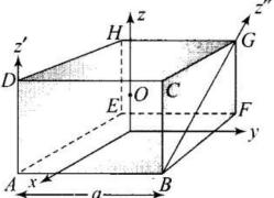
**Sol:** (b, d) We can apply the concept of symmetry to calculate the net moment of inertia. Moment of inertia about two symmetrical axes are same.
