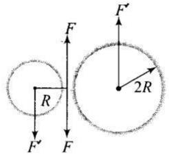
(c) Let  $_{\rm I}$  and  $_{\rm 2}$  be final angular velocities of smaller and bigger drum respectively (anticlockwise and clockwise respectively).
