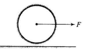
**Sol:**In this problem friction force on the disc will act in opposite direction of F at the point which in contact with surface at any instant of time and supports the rotation of the disc in clockwise direction.
