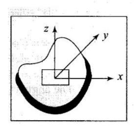
The sum of moments of inertia of a laminar object about two mutually perpendicular axes lying in the plane of lamina is equal to the moment of inertia about an axis normal to the plane of the lamina and passing through the two perpendicular axes. This theorem is applicable only for laminar (thin sheet kind of) object.
