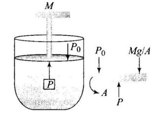
As the pressure remains constant, so if the temperature is increased, only the volume increases as the piston moves up without friction.
