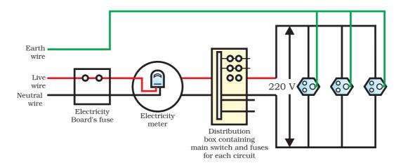
A fuse in a circuit prevents damage to the appliances and the circuit due to overloading. Otherwise the appliances or the circuit may get damaged.
