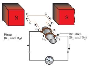
**31.** Explain working with the help of the diagram. To get a direct current a split ring type commutator must be used in place of slip ring type commutator.
